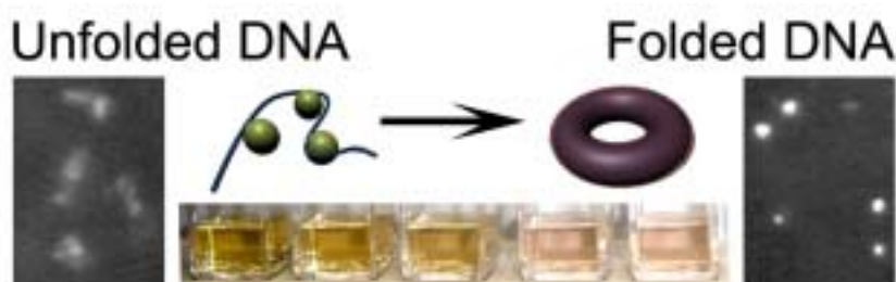
Figure. DNA high-order structure can be detected through metallization by noble metal (picture shows the example of silver metallization) at a very low concentration ( 10^{-9} g/L).
