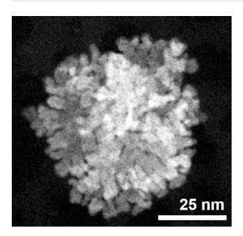
The alloy catalyst of ruthenium and iridium, which measures 60 nanometers wide (one nanometer is one-millionth of a millimeter), looks like coral in a microscopic image. (Provided by Kyoto University)
